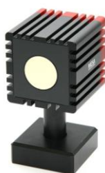
Fig. 4: SwissRanger SR4000 ToF Sensor.
